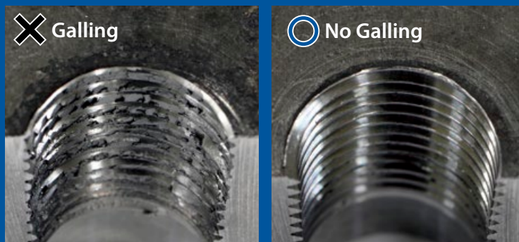
SS400材での加工イメージ Image to process taper pipe thread in SS400 material
